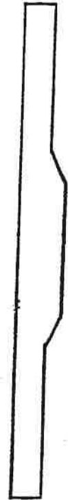
Figure 6 50 foot passing lane is 18 feet wide with 12.5 foot long entrance and exit triangles.
